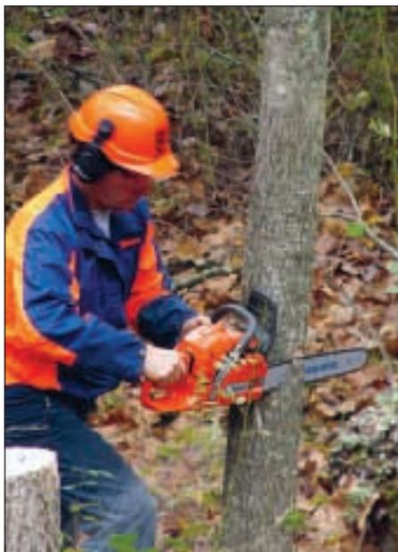
*Make the top cut first when making the face notch. Line up the top cut using the felling sites provided on today's professional chain saws.*
