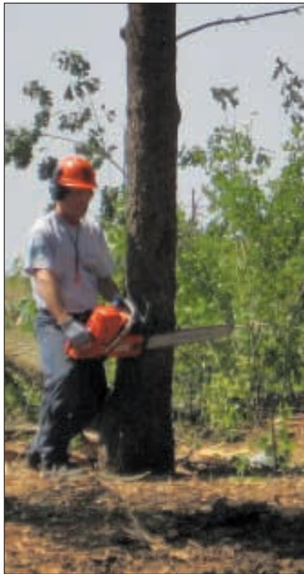
*Line up the top cut while bracing your body against the tree and facing the desired felling direction.*
