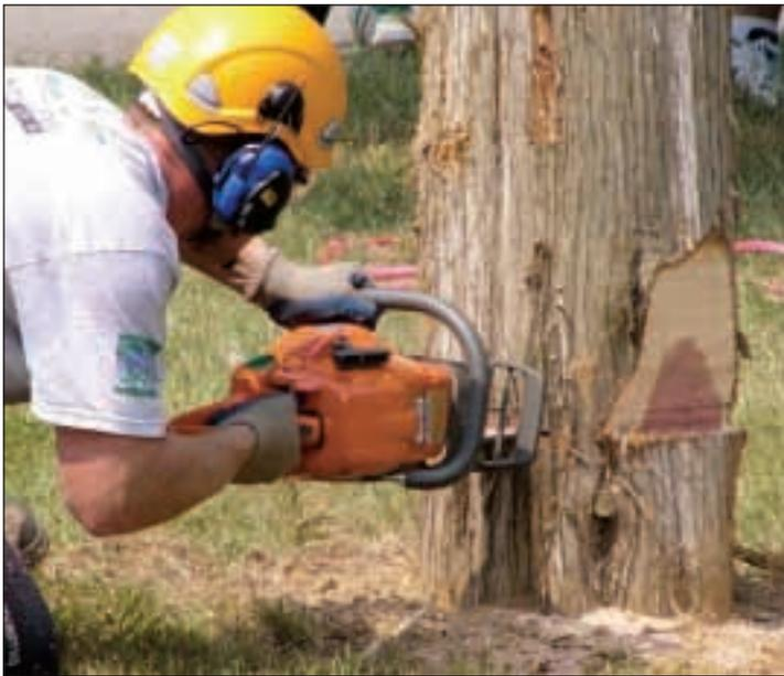
*The bore cut is another way of making the back cut and establishing the hinge, reducing the chance of “barber chairing” and establishing the hinge while the tree stays locked on the stump by the back strap.*
