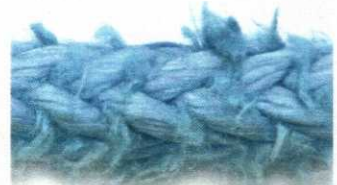
Severely abraded rope.
