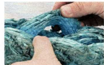
Inspect for pulled strands.
